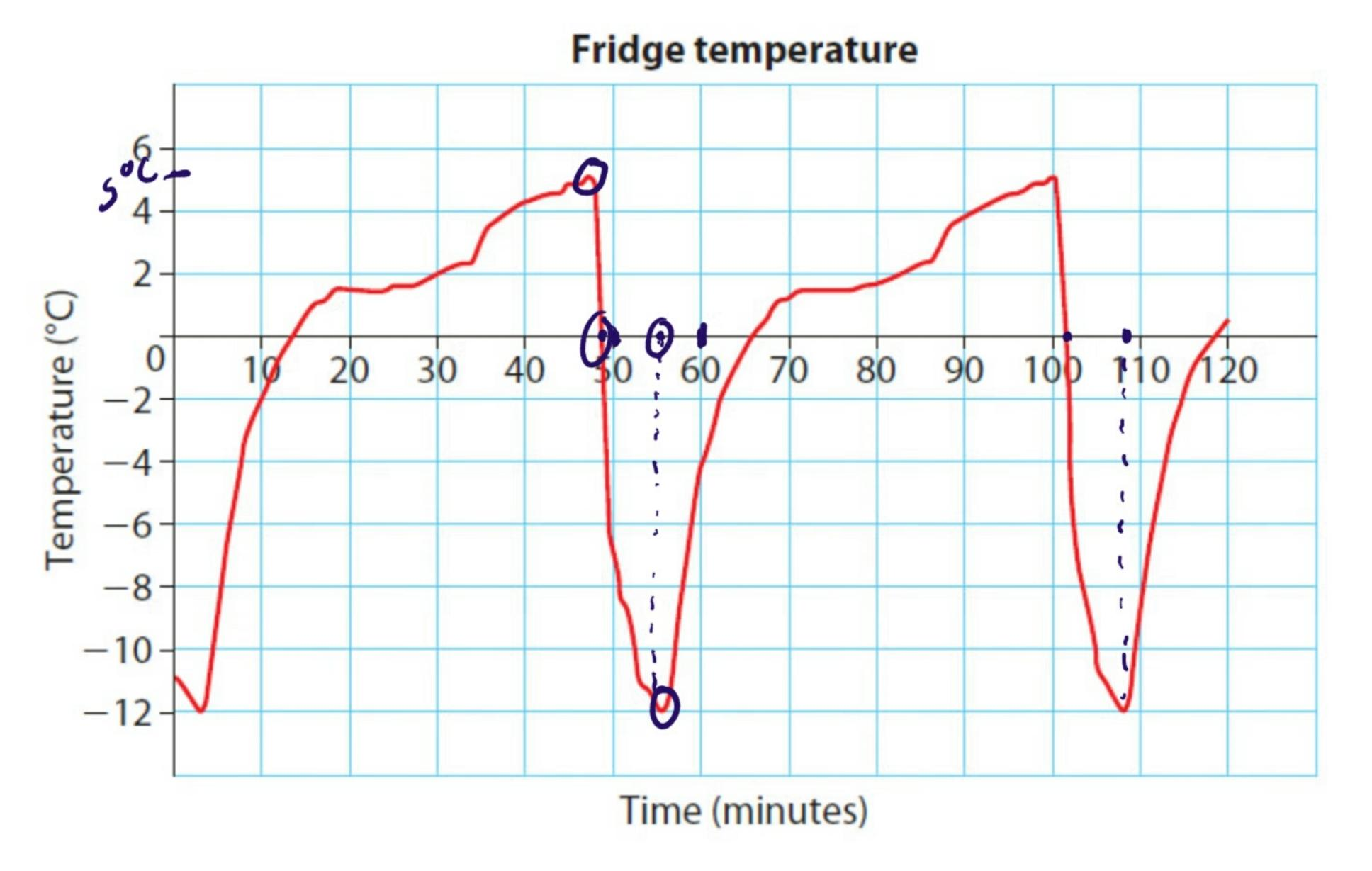
The fridge has a motor which cools down the inside. The motor is switched on and off by a thermostat.
